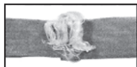
Holes/tears/cuts in cover; exposed/damaged yarns
